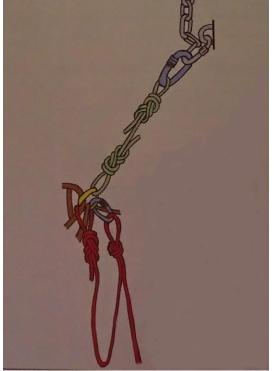
Then take some slack on your rope, make a knot and tie it to your belay loop (and not to loop. At this point you're still secured cordelette) fixed on your belay loop <u>a gear loop</u>) using another screwgate carabiner. The point of this step is to prevent from losing the rope and to stay on should never put you off belay ! belay from your belayer on the ground.
