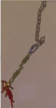
First, tie on to the chain belay with a sling (or better with a 9mm and a screwgate carabiner.
